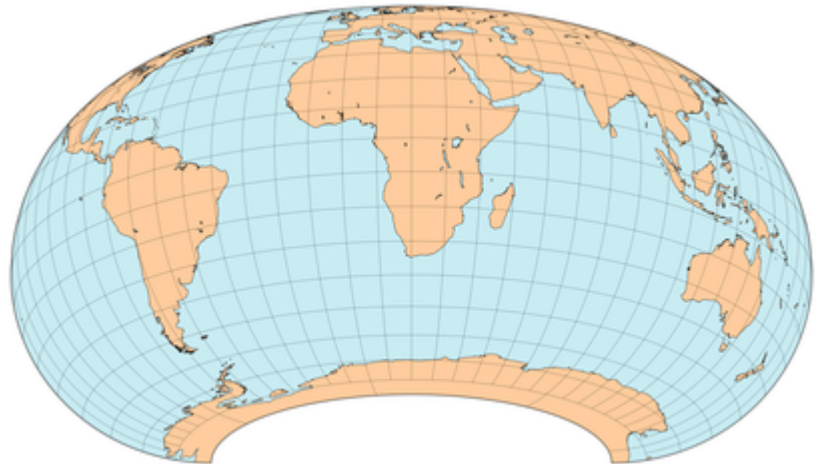
Armadillo map emphasizing the southern hemisphere: tilt angle 20°, central meridian 20°E, no repeated portions.
